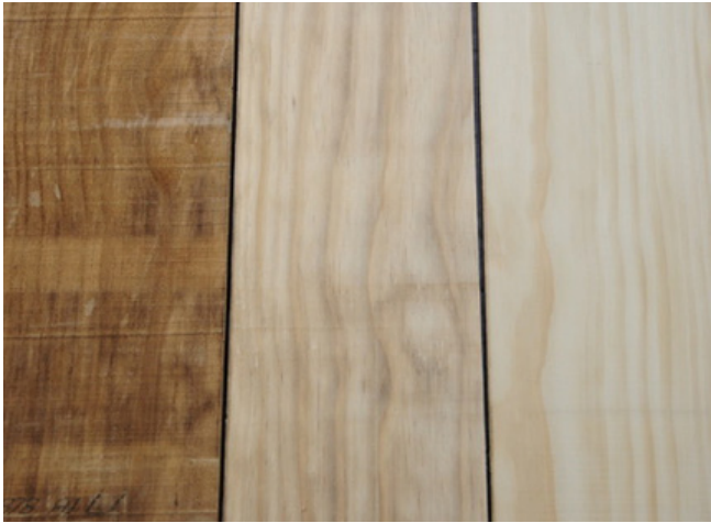
DISCOLORATION: ROUGH BOARD, AFTER SURFACING 1/8 INCH AND AFTER SURFACING 1/4 INCH FROM ROUGH
