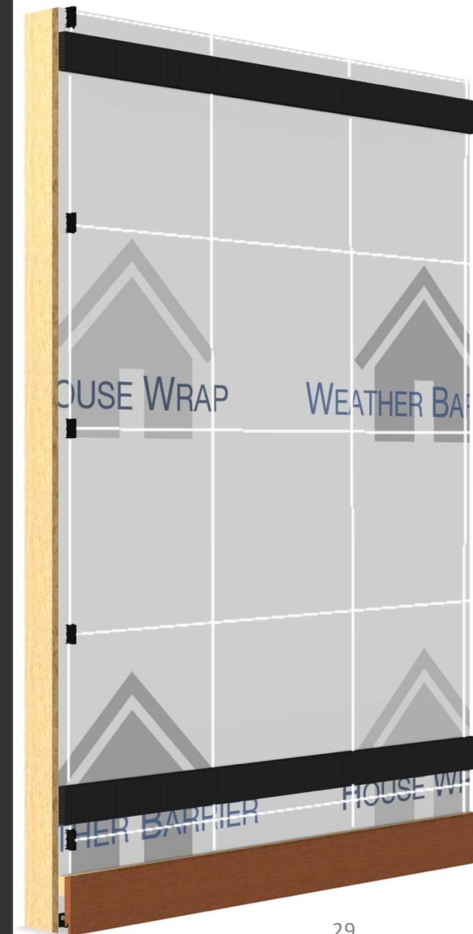
Step 14: Insert your first vertical board into the column of clips, gently tapping with rubber mallet if necessary.
