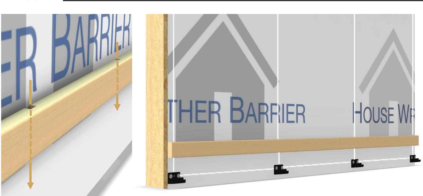
**Step 8:** Fasten the furring strip across the length of the wall above the installed starter clips to the appropriate height that matches the width of the trim board. Ensure the furring strip is installed into the framing.
