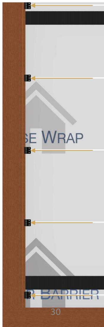
Step 16: Continue to install clips and Rainscreen boards until you have covered the span of your installation area. Clips will usually require only one screw each at this point of installation.
