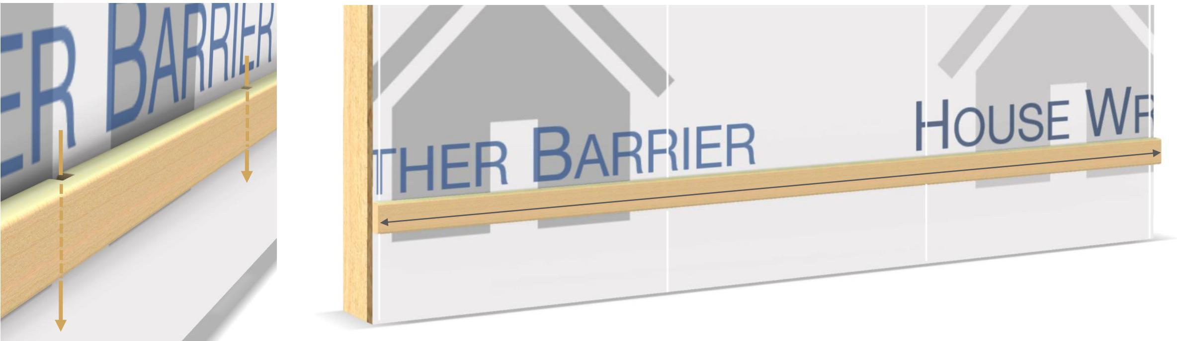
Step 4: Obtain enough length of 1 x 2" furring strips to cover the entire length of the wall. Cut small vertical channels (weep holes) into the furring strip approximately 12 inches apart. These are required to allow for drainage through the furring strip. These channels will face the wall.
