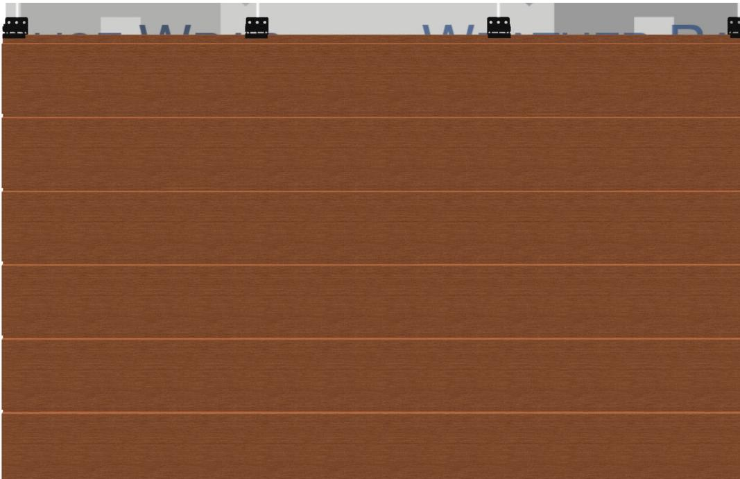
**Step 9:** Once the clips are engaged, install the second set of clips, driving one or two screws through the siding fastener into the stud. Ensure that the clips are level, and continue to check level throughout the installation.
