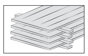
flooring doesn't need to be acclimated as long as a solid floor, it is still advisable to bring the flooring up to the approximate temperature and humidity to be expected in the space. Unbundle your flooring and stack each plank so that air is able to circulate through the stack. Thus, acclimating each piece to it's new environment.
